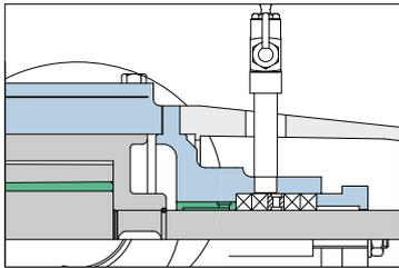
Sealing with stuffing box, with or without lantern ring, for use of external lubrication. Used for high viscosities and where some leakage is allowed.
