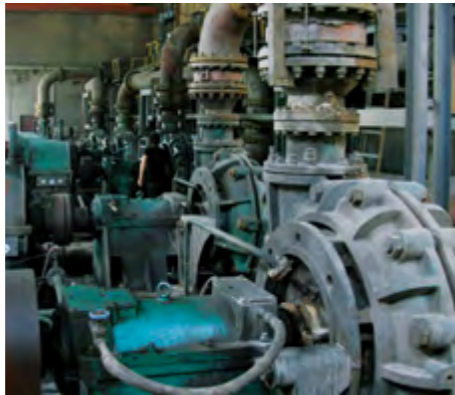
Two 150ZGB high head slurry pumps in series pumping coal tailings direct from a thickener underflow.
