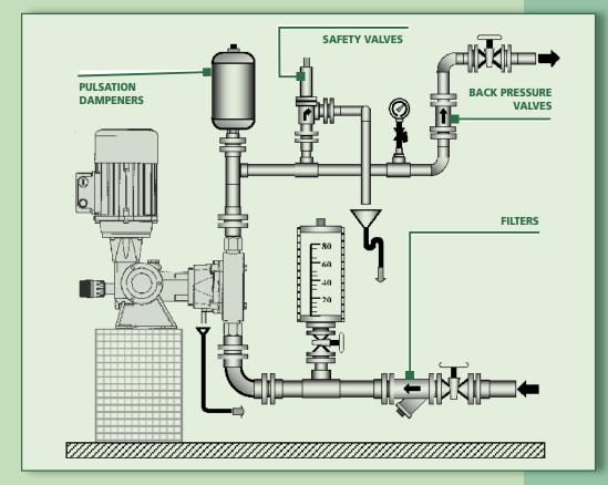
Each metering pump can be supplied with accessories in order to improve the operation and accuracy of the units.
