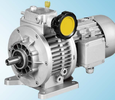
MV Series Variable Speed Driver Speed Range : 200 - 1000rpm Torque: 0.003 - 0.352kN . m Power: 0.37 - 22kW
