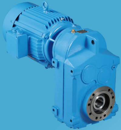
F Series Parallel Shafts Helical Gear Units Ratio: 4.3 - 273 Torque: 0.11 - 18kN .m Power: 0.12 - 160kW
