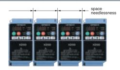
Side-by-side installation has derating for carrier frequency and output current required
