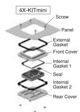
You can mount an optional keypad with the potentiometer part no. OPE-SRmini for a NEMA1 rated installation. The kit also provides for removing the potentiometer knob to meet NEMA 4X requirements, as shown (part no. 4X-KITmini).
